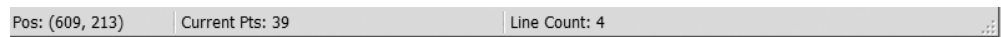
Figure 6.2 A sample status bar with the fields getting 1/6, 2/3, and 1/2 of the total width
