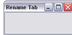
Figure 6.3 A form with a fixed size and border style set to FormBorderStyle.FixedDialog
