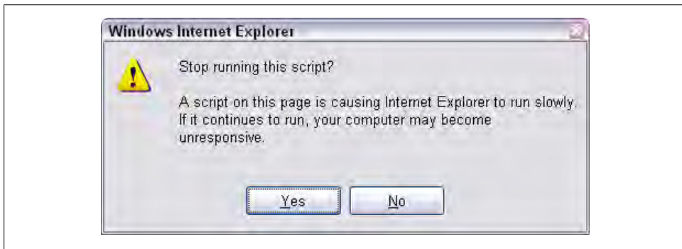
Figure 6-2. Internet Explorer's long-running script warning dialog is displayed when more than 5 million statements have been executed
