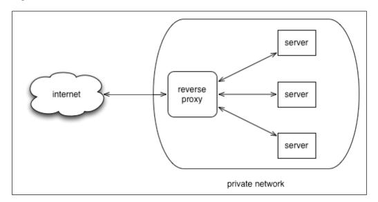
This is the type of proxy we can use to balance requests from clients across many Node servers. Client X does not communicate with any given server directly. A broker Y is the first point of contact that is able to direct X to a server under less load, is located closer to X, or is, in some other way, the best server for X to access at the time.
