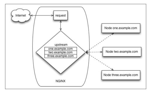
Each request will be handled first by Nginx, which will check its *upstream* configuration and, based on how it is configured, will (reverse) proxy requests to upstream servers that will actually handle the request.
