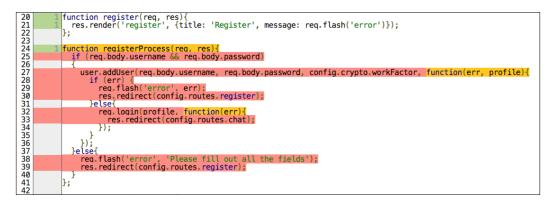
Green means executed, red is not executed, and yellow is a function that has not been tested. Once we are using code coverage, identifying our next test becomes easy. We find a file, require it in a test, look at all the lines highlighted in red in the file, and slowly create tests until all the red highlights are gone.
