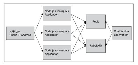
The front public-facing address of our site will be the server that is running HAProxy. In this setup, we will only want one server running HAProxy, and if it is production, this site should have a static IP and a public DNS record. HAProxy is very efficient at load balancing, and one of them can handle a lot of traffic. Eventually, we can run two behind a balanced DNS record, for example, but this is out the scope of this book.
