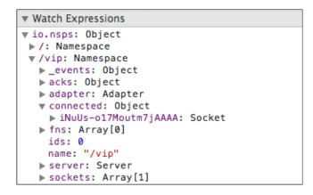
We can see that each attribute of this object ties to a namespace. There is the default namespace and the /vip namespace. I have expanded the /vip, so you can see its attributes. The two attributes of note are the name, which is the string that we pass in when we first create it (io.of('/vip')), and the other is the connected object. This has all our sockets that are currently connected. The connections are mapped based on their socket ID.
