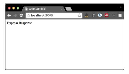
In order to receive this response, the app.get function uses a regular expression to match any GET request, no matter the path. The req and res objects are the request and response objects. The res.send Express function adds all the basic headers for us, before sending the response back.
