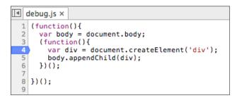
Reload the page and processing should stop at line **3**. From here, we can resume execution, step over, step into, and step out, as shown in the next screenshot:
