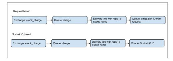
We can see that both versions start the same way. This is important to remember, as we want a reusable exchange and queue to start this process. Once the credit card has been charged, we divert, as each one will respond to different queues. This allows us to have one worker but many unique response queues.
